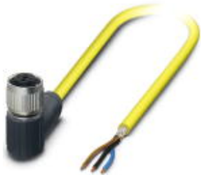
Sensor/Actuator cable, 3-position, PVC, Yellow RAL 1021, shielded, Free cable end, on Socket angled M12-SPEEDCON, A-coded, Cable length: 2 m
